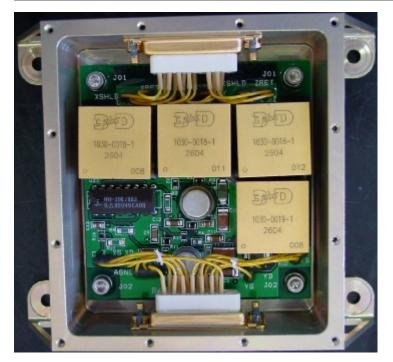
**Fig. 6** Preamplifier box. The 3 upper cubes correspond to the 3 antennas preamplifiers, the fourth one is for power regulation. They are manufactured in 3D technology . The electronics for the in-flight calibration is also shown on the PCB. The preamplifier box size is 95 mm x 81 mm (109 with the mounting  $\frac{1}{2}$  ears  $\frac{1}{2}$ ) x 30 mm
