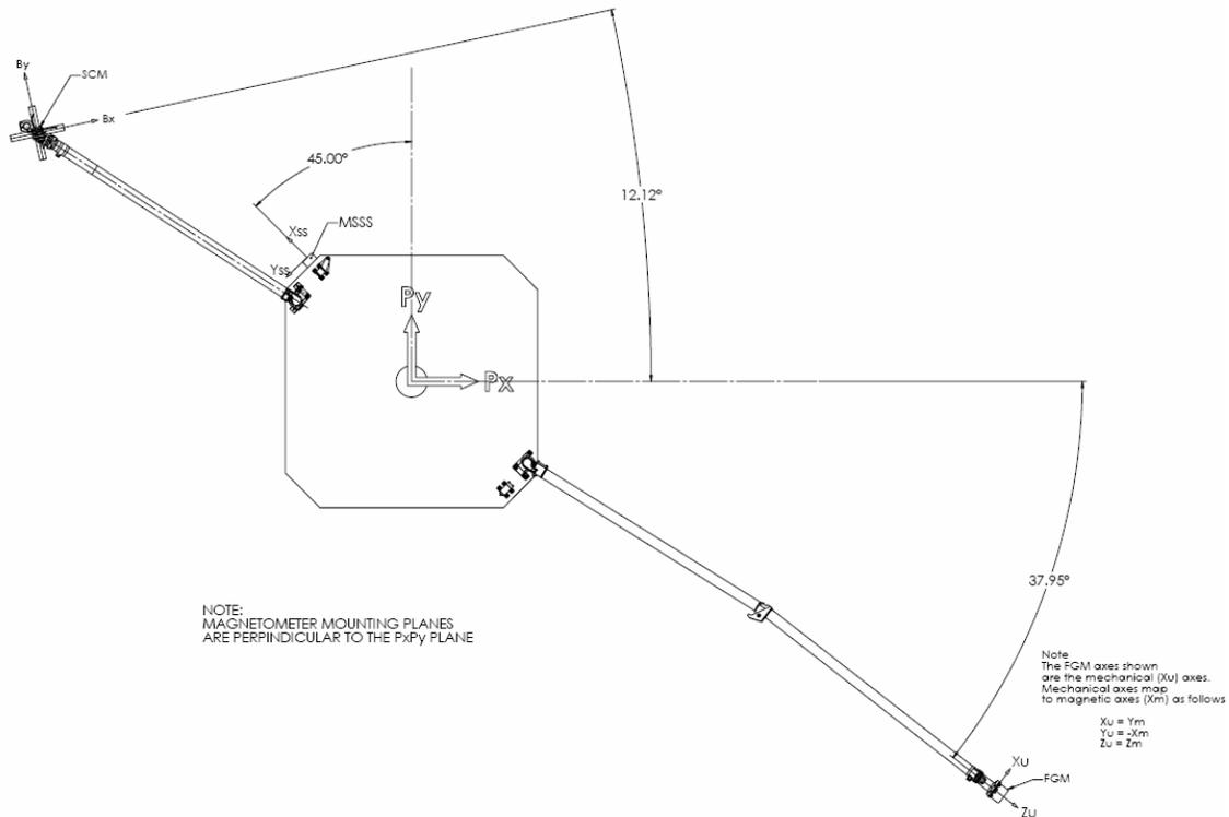
Figure 19: Accommodation of FGM sensor on boom
