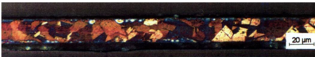
Figure 1: Metallographic microstructure of the 13Fe-81-Ni-6Mo alloy annealed at 850°C (after Müller et al., 1998)
