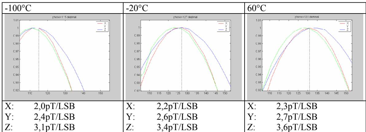
Figure 14: Input sensitivity and phase of ADC sampling versus excitation clock in dependency on sensor temperature. Upper panel show the sensitivity versus phase angle, the numbers below provide the sensitivities absolutely
