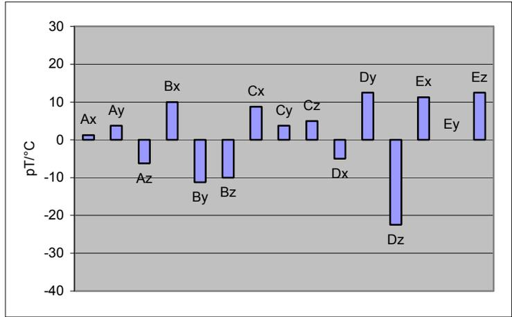
Figure 11: Offset drift of all sensor components (Probe A-E) caused by excitation and pick-up electronics in dependency on electronics temperature
