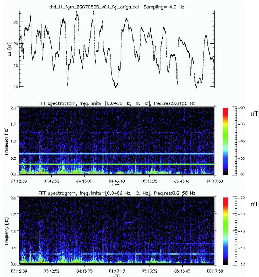
*Figure 23: Data before and after correction of interferences induced by the power supply. Upper panel: time plot of the spin axis component. Central panel: dynamic spectra of original spin axis data. Bottom panel: dynamic spectra of spin axis data after applying the correction using the sun pulse triggered interference model. The FFT's are calculated using 128 4Hz samples*
