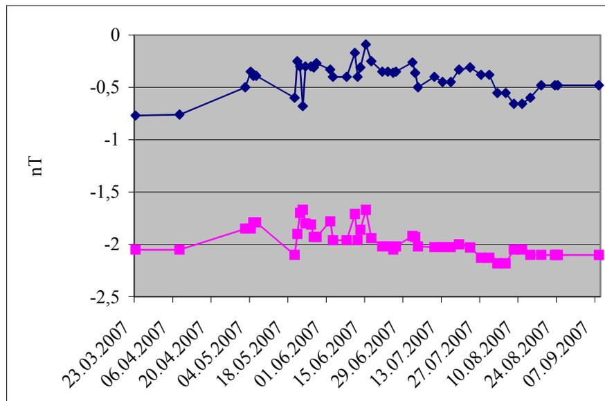
Figure 21: Offset of Probe A spin plane components in the first half year of flight
