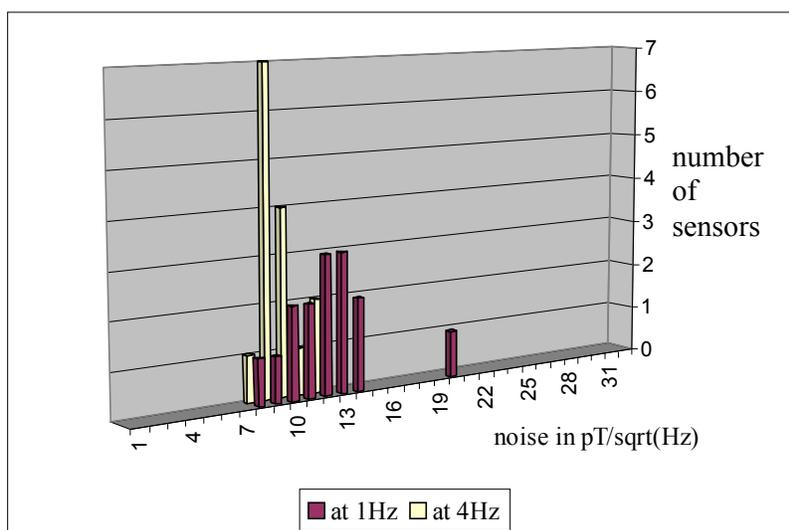
*Figure 20: Noise Statistic measured inflight: The overall noise was measured for each sensor at quiet field conditions. The sensors are sorted by noise levels at 1Hz and 4 Hz. A noise level less than 30 pT/Sqrt(Hz) at 1Hz was required*
