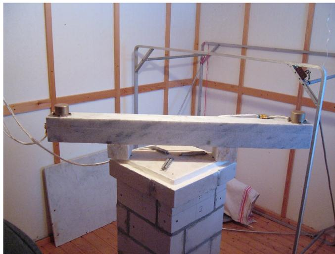
*Figure 17: Two Themis sensors mounted on a pillar to measure Earth field components for comparison with an observatory instrument*
