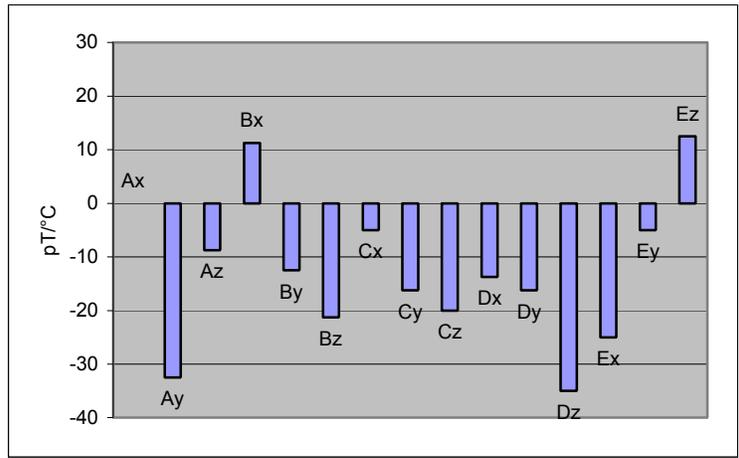
Figure 12: Offset drift of all sensor components caused by feedback circuitry in dependency on electronics temperature
