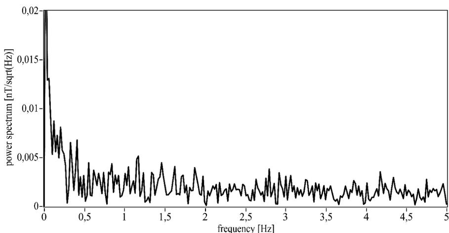
Figure 2: Noise spectrum of a 13 mm ring-core as used for Themis
