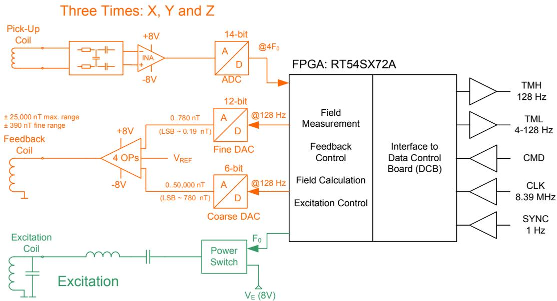
Figure 4: Block diagram of the FGM sensor electronics
