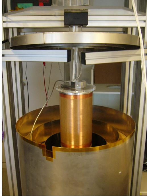
*Figure 10: TCU with coil system and sensor rotation capability*
