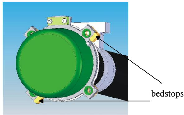
*Figure 8: Sensor fixation on boom for repeatable sensor mounting*
