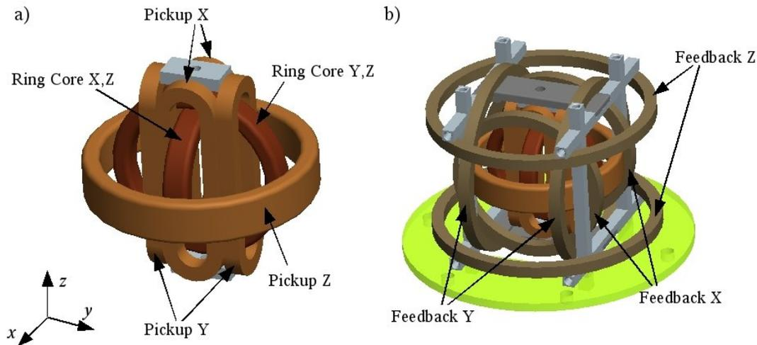
Figure 3: 3-D model of the FGM sensor with a) ring cores and pick-up coil system and b) fully functional sensor including the Helmholtz feedback system
