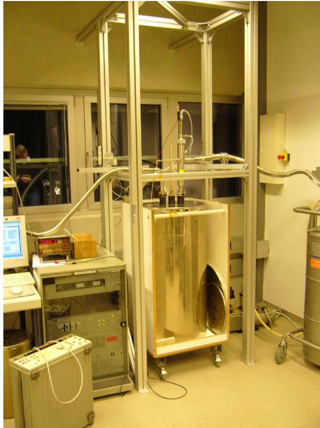
Figure 13: Facility to measure the dependency of instrument parameters on sensor temperature
