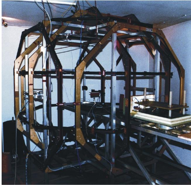
*Figure 16: Coil system with thermal box baseplate in Magnetsrode, Braunschweig*
