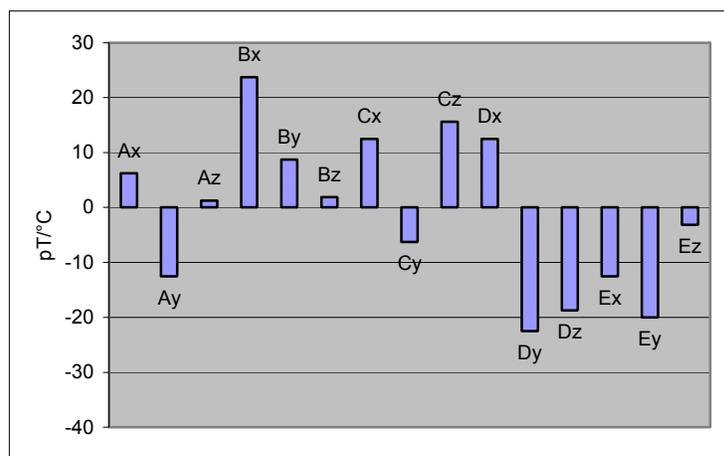
Figure 15: Offset drift of all sensor components caused by the sensor in dependency on sensor temperature
