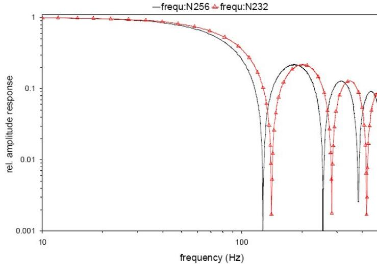
Figure 9: Amplitude response of 128 Hz data
