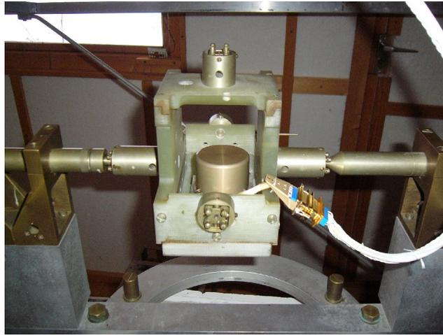
*Figure 7: Sensor in fixture which defines the mechanical reference system with a precision of 10 arcsec*
