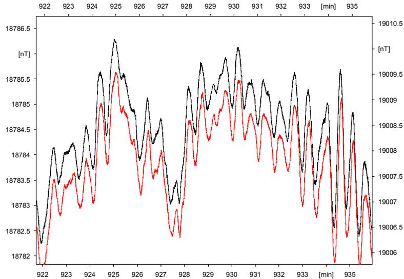
*Figure 18: Pulsation measurement of two Themis magnetometers performed in north-south direction of the Earth field. Field variations measured with an independent observatory instrument confirm the result of both Themis magnetometers*
