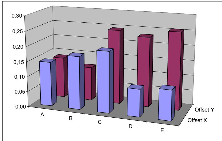
Figure 22: Offset variation (standard deviation in nT) of spin plane components of all five Probes
