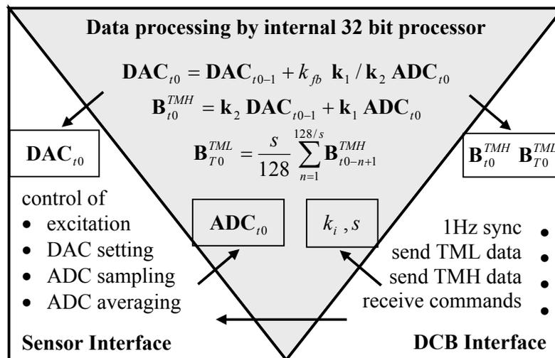
Figure 5: Block diagram of the magnetometer FPGA
