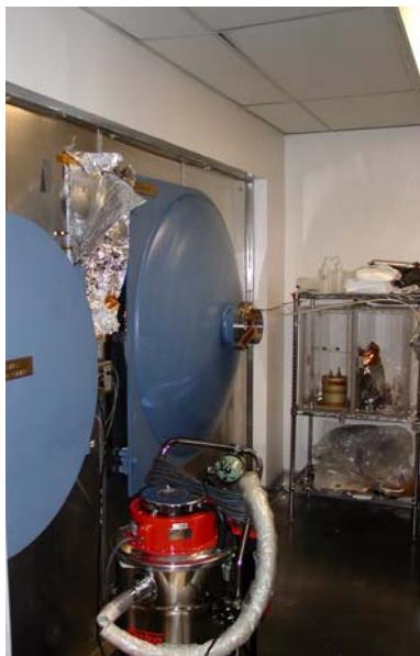
Figure F-51. Large T/V chamber to be used for full instrument complement thermal cycling.
