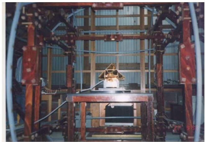
Figure F-53. SCM calibration facility of CETP.
