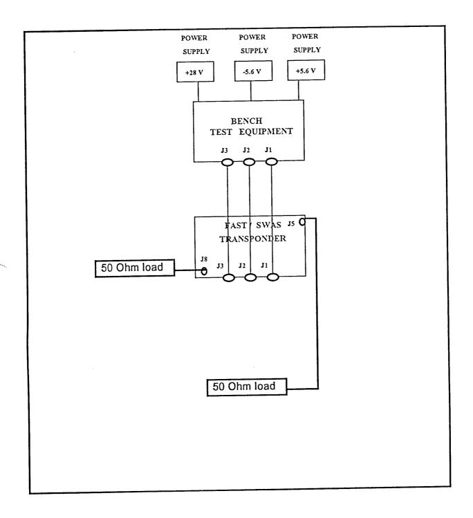
Fig. 1.0 Transponder test set block diagram
