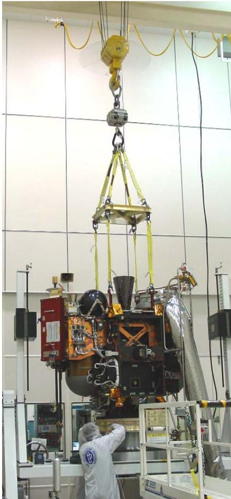
Figure 3. Spacecraft, lift fixture and crane prior to separation from integration fixture.
