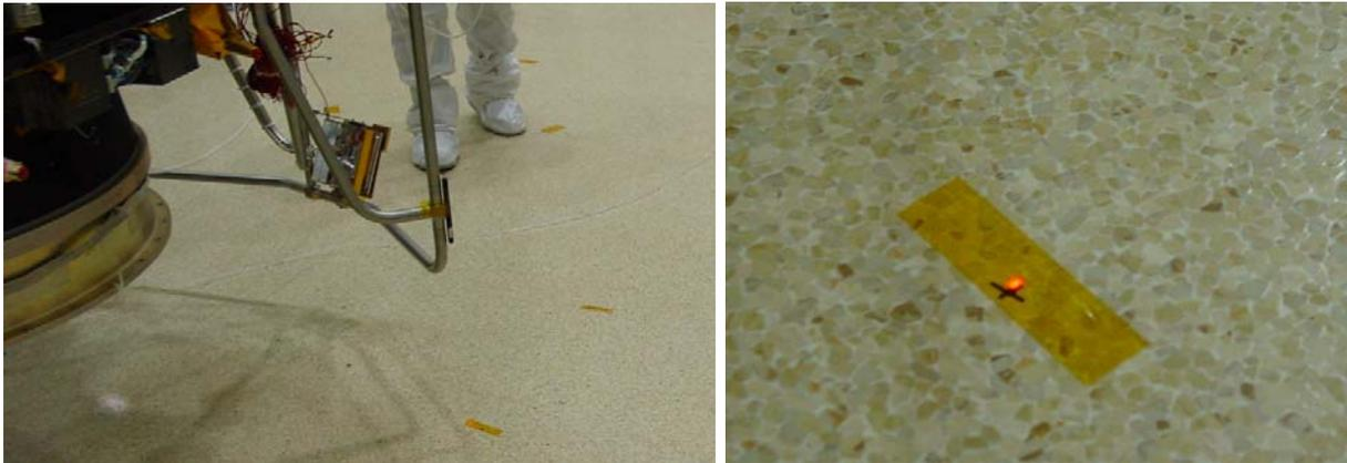
Figure 9. Reference laser pointer and spot used to locate and reproduce equilibrium positions and displacement prior to release for pendulum swing motion.
