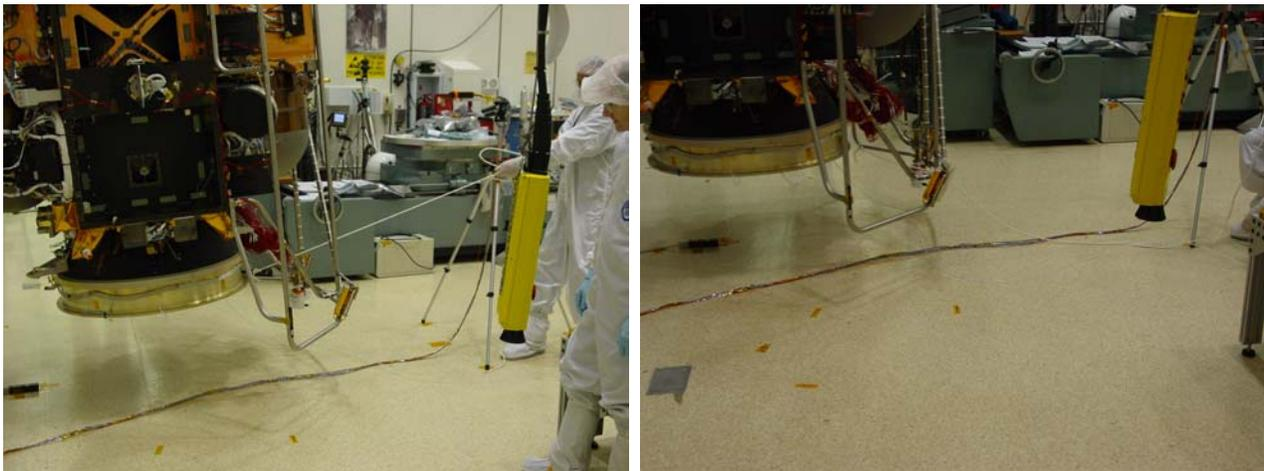
Figure 12. Displacement of the spacecraft in the  $+X_S, -Y_{SC}$ , South direction (left) and about 1 second after release during the free pendulum motion (right).
