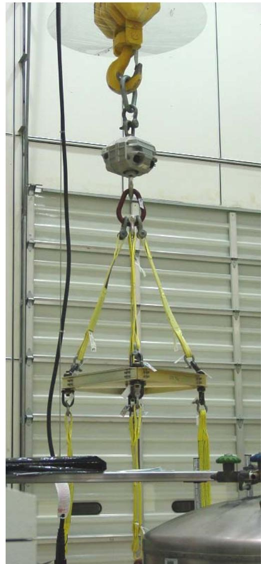
Figure 2. Spacecraft lift fixture and crane hook.
