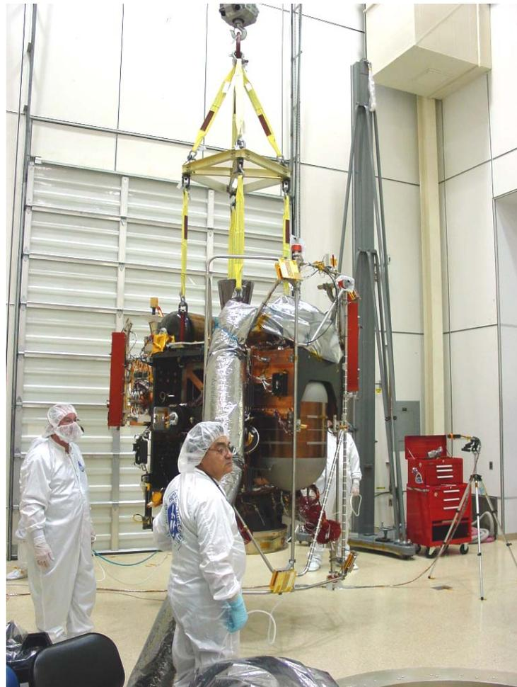
Figure 4. Spacecraft suspended from lift fixture at the North end of high bay. Test magnetometer and tripod can be seen to the right (East) of the spacecraft.
