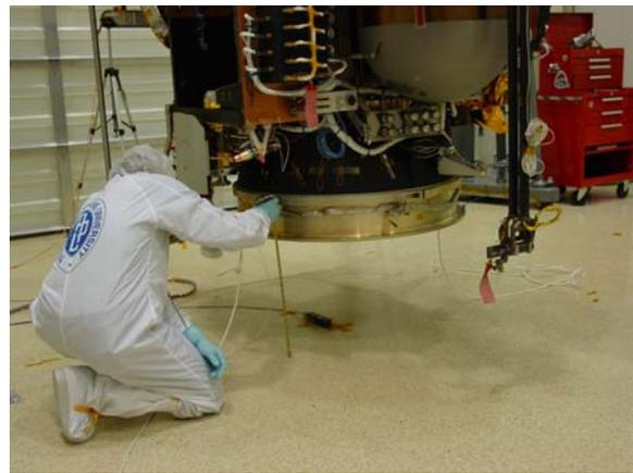
Figure 8. Measuring the height of the spacecraft adapter fitting above the floor. MAG-FLR can be seen underneath the spacecraft.
