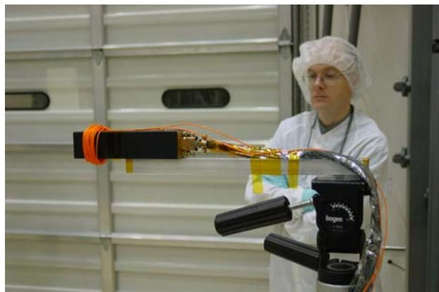
Figure 6. Field-test magnetometer B mounted on a camera tripod. The magnetometer is the black rectangular box at the left upper end of the aluminum box channel. The orange wire windings provide a timing signal in the magnetic field data stream.
