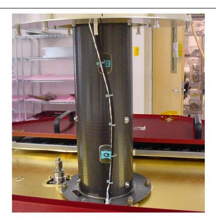
Staking material will be reapplied where the coax passes through the AXB flange and deck. This routing provides enough room for the FGB and the blankets. Swales should dress the harnesses in this fashion on the remaining probes.
