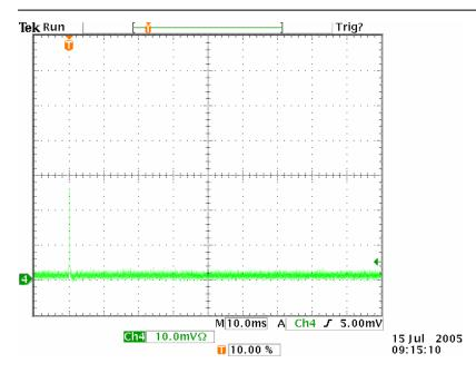
This plot shows a 1.3Amp inrush when turning on the HV FETs on the ESA HV Motherboard. This will also cause the PCB to trip off the ESA supplies. This was the problem that was observed in Thermal Vacuum.
