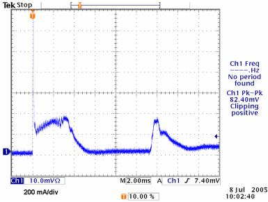
The profile includes 2 current spikes where the second current inrush ended approximately 15ms after turn on. The PCB can only ignore transient inrush for about 9-10ms. With the inrush at around 400mA and 12ms after turn on, the PCB will certainly trip off because the current threshold is set to 250mA.
