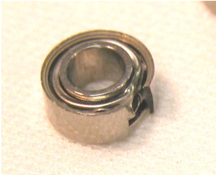
Picture 1: Bearing Failure, Part number SR144ZZMC3 3GM6 (Inner Bearing of Assembly)
