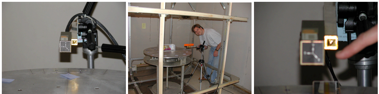
Figure 5. The magnetometer was positioned on an aluminum box channel mounted to a tripod. The level of the magnetometer was adjusted to better than 0.5^\circ and one corner of the magnetometer was chosen as the reference point.
