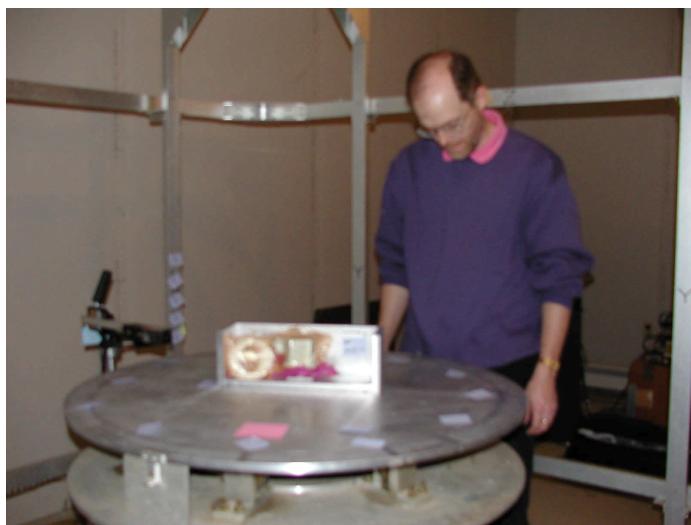
Figure 6. Rotating the table in 30^\circ increments, waiting approximately 5 seconds at each step, constitutes one 'run'. Measurements for a given valve consisted of six such runs.
