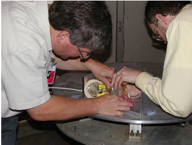
Installing a valve in test fixture
