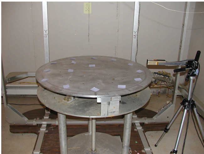
Non-magnetic turntable & miniature magnetometer
