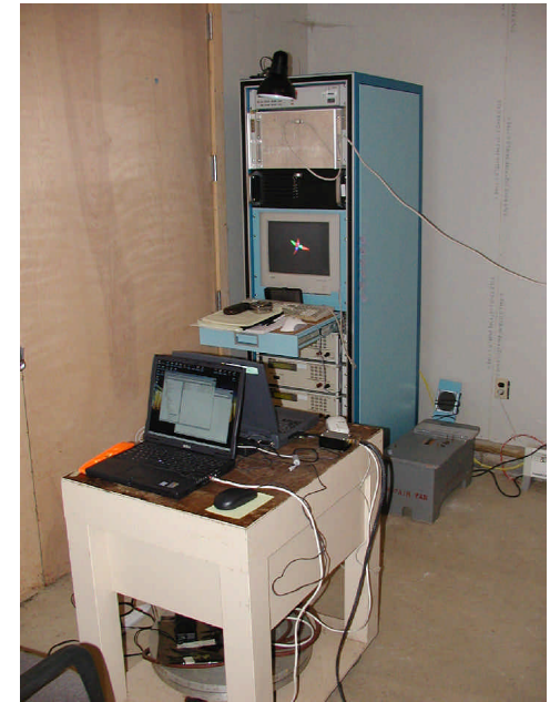
Control electronics: coils, test magnetometer, analysis computer
