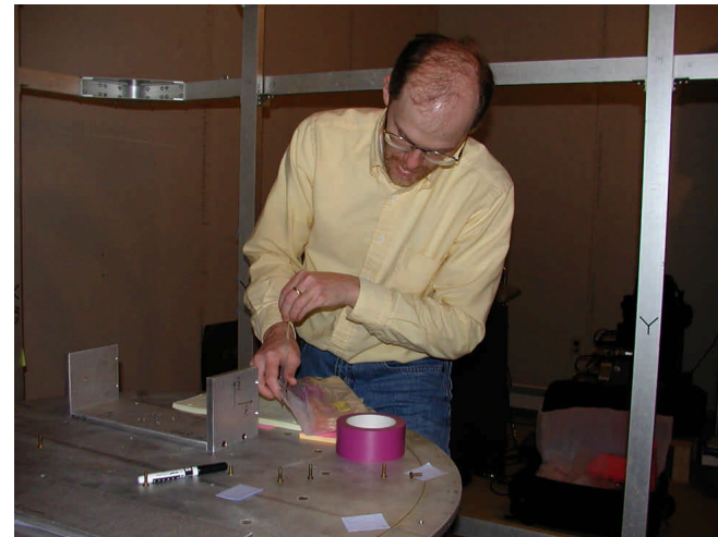
Valves wrapped to stay clean w. mount exposed
