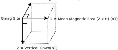
H-Axis points towards the approximate mean magnetic north as measured from installation site during quiet time.
